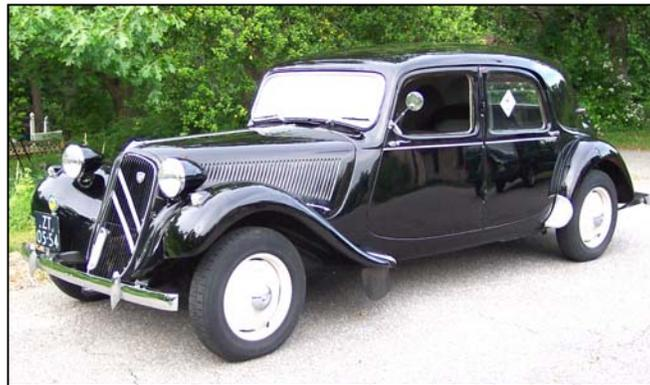
**Dave Phillips' 1954 Citroen Traction Avant. This is the mid-level model known as the Normal. It has a 1.9L, 56 HP, four-cylinder engine, three-speed transmission, front wheel drive, and 121-inch wheelbase. This classic design dates back to 1934 – production ended in 1957.**
