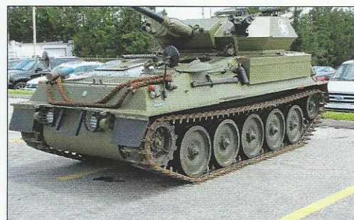
According to the owner, Paul Winicki, the above military vehicle is a 1978 Alvis Scorpion. Engine in the Scorpion is a Jaguar J60, 6-cylinder gasoline motor generating 190 horsepower (later replaced by a Cummings diesel-fueled 190 horsepower engine).
