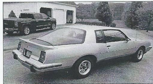
Since the enormous rear glass is fixed (not an opening hatch), it forced adoption of a dramatically shortened trunk opening.
